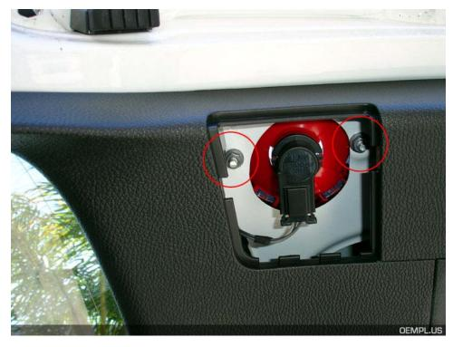
1.3 To disconnect the wiring harness, you will have to release the two small retaining tabs. This can be done by squeezing them and rocking the connector back and forth until it comes loose.
